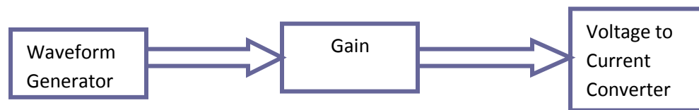
Figure (3.2): Block Diagram of Signal Generator
