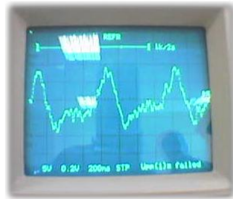
Figure (4.1): The ICG Signal from Hardware Circuit
