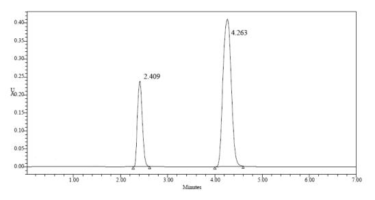
Fig.No.3: Chromatogram showing standard
