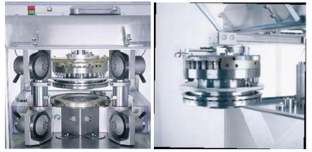
Figure 8: Xpress® 700 tool free turret removal system
