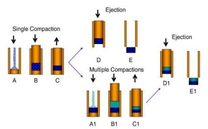
**Figure 6:** Schematic Diagram Showing The Manufacture Of Single And Bilayer Tablets Utilizing Uniaxial Compaction. A- Die Filling, B-Compression, C-Decompression, D- Lower Punch Removal And Reapplication Of Load To The Upper Punch, E-Tablet Fully Ejected. 1 Refers To The Final Compaction Conditions
