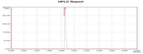
Figure.2 Chromatogram of standard solution
