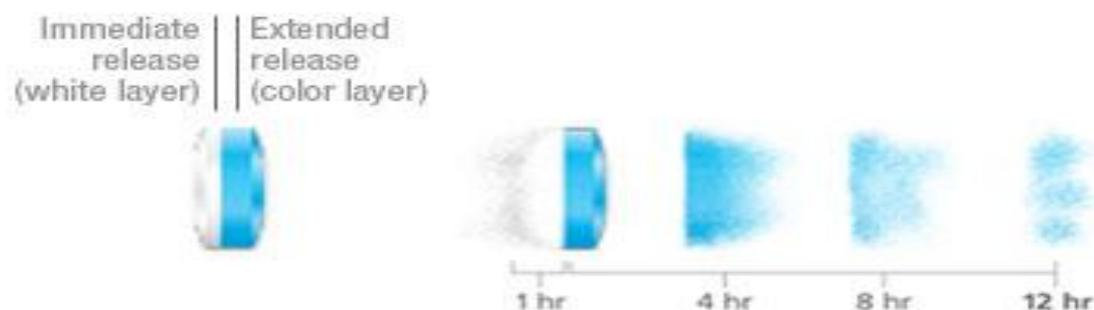
**Figure 1:** Drug release mechanism of a bilayered tablet comprising an Immediate release & a Sustained release layer
