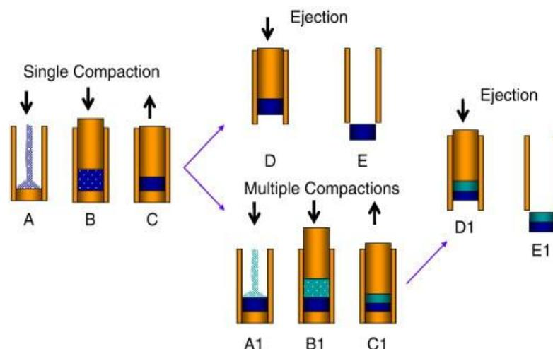
**Figure 6:** Schematic Diagram Showing The Manufacture Of Single And Bilayer Tablets Utilizing Uniaxial Compaction. A- Die Filling, B-Compression, C- Decompression, D- Lower Punch Removal And Reapplication Of Load To The Upper Punch, E-Tablet Fully Ejected. 1 Refers To The Final Compaction Conditions
