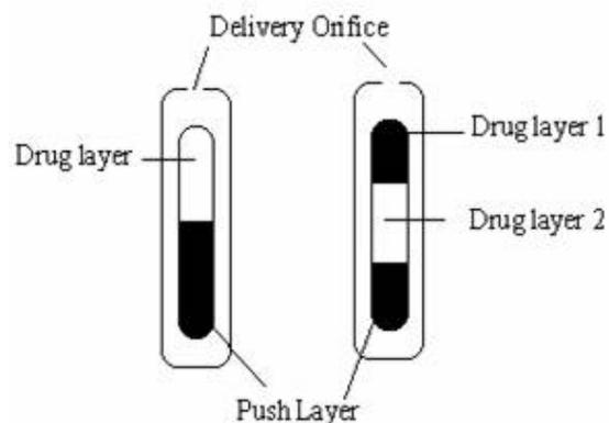
Figure 2: Bilayer and trilayer OROS push pull technology
